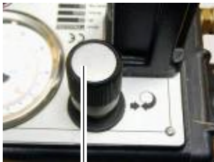
adjustment pressure valve
